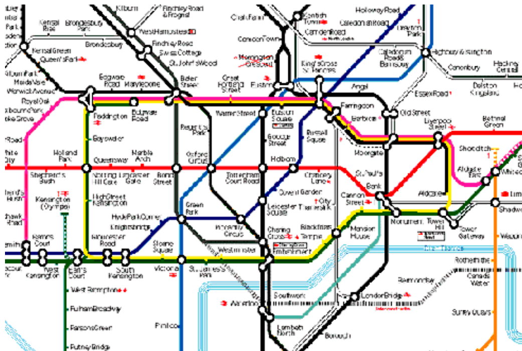
Figure 1. The London Underground Schematic: an example of a geoschematic. The geographic relationships between nodes (stations) in the network have, generally, been maintained. The edges (lines) in the network have undergone significant transformation (e.g. straightening etc.).
