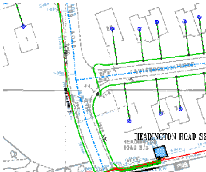
Figure 3. A geographic view part of a LV network, supply points on an LV network, HV network and a substation (Headington Road SS).
