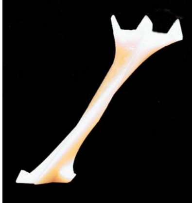
Figure 5. Wax model generated by a rapid prototyping machine at the Sagrada Família from the digital model
